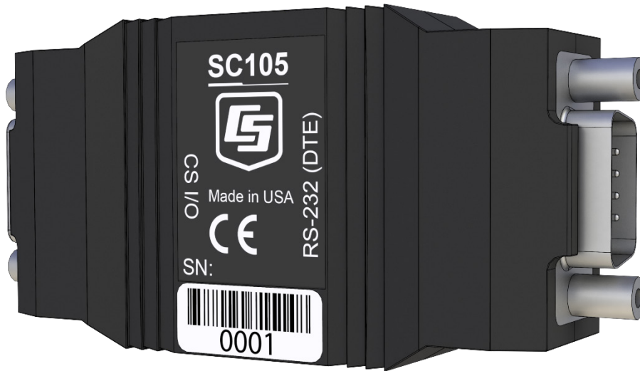
FIGURE 1-1. SC105 CS I/O to RS-232 Interface
